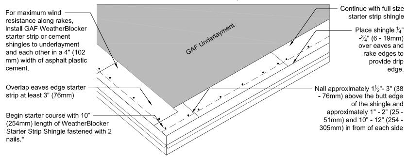
\* NOTE: For all applications, the butt joints of the WeatherBlocker™ Starter Shingle must be offset from the butt joints of the first course of shingles by 4" or more. For long eaves, a 10" (254 mm) piece of Weather Blocker™ Starter may need to be installed periodically to adjust the offset. The frequency of this adjustment will depend on the length of the shingle being installed.
