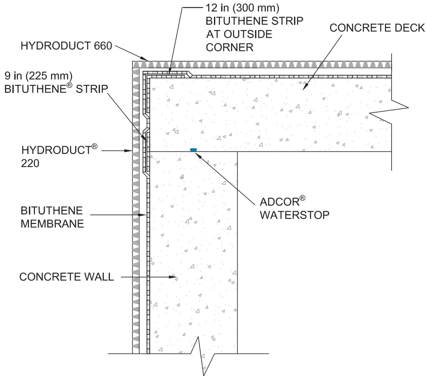
NOTE - GCP MAY REQUIRE AN ALTERNATE GCP WATERSTOP BASED ON DESIGN CONDITIONS
