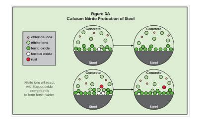
Second, the nitrite anions chemisorb at the iron surface and create a fortified ferric oxide protective layer. As in Figure 3B, the nitrite ions enhance the natural protection provided for steel by concrete. As shown in Figure 3C, ferrous oxide defects are surrounded by nitrite ions, and less likely to be exposed to chloride ion attack.
