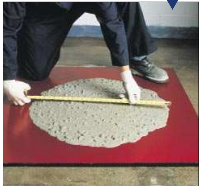
Slump Flow Test to measure slump diameter
