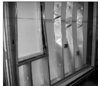
*Grace air barrier systems withstood wind gusts equivalent to 168 mph, remaining fully adhered and intact while substructure was brought to failure.*
