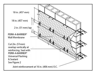
PERM-A-BARRIER<sup>®</sup> Wall Membranes must be protected from damage by other trades or construction materials.
