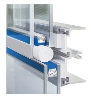
EdgeSil IGS3760 is EOTA category 1 approved to support façade system designs based on inserts in the edge seal of the insulating glass unit.
