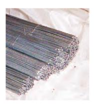
• Straight cut 12 gauge soft galvanized wire.
