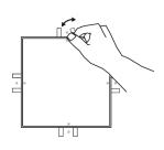
Place fasteners as shown and secure with drywall screws 3/4" from the edge.
