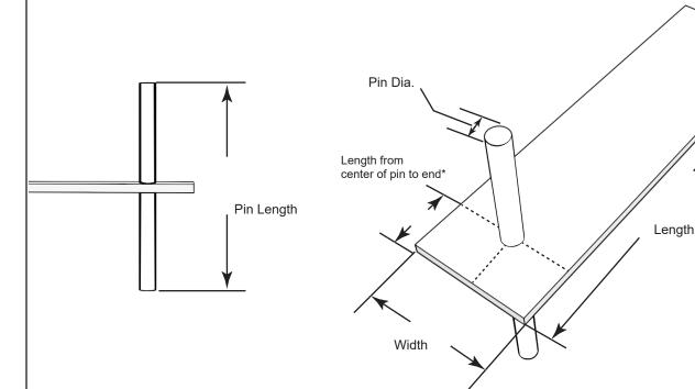
\*Pins are available loose or welded in place.
