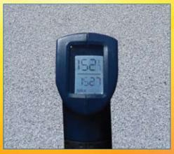
Uncoated white granulated roof = 152°F
