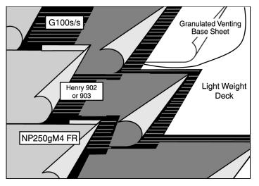
modifiedPLUS® NP 250gM4 FR Cap & Cap Flashing modifiedPLUS® Base Sheet Flashing modifiedPLUS® Base Sheet G2 Granulated Venting Base Sheet Lightweight Concrete Deck
