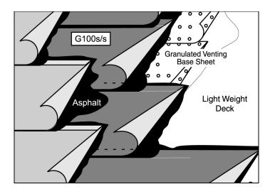
modifiedPLUS® NP 250gM4 FR Cap & Cap Flashing modifiedPLUS® Base Sheet Flashina modifiedPLUS® Base Sheet G2 Granulated Venting Base Sheet Light Weight Concrete Deck
