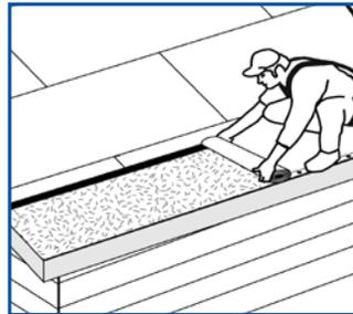
Cut rolls in half and allow to lay flat to relax for 20 minutes. Align at eave.
