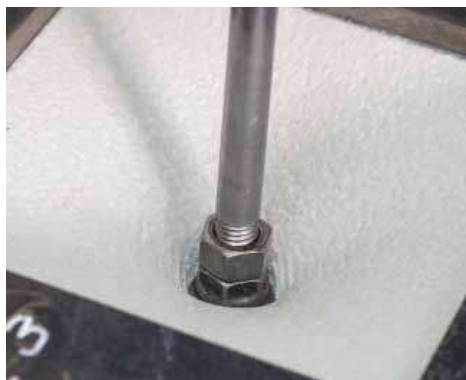
Pliable MiraPLY-H with SeamLOCK™ Technology inherently absorbs impact during a puncture test.
