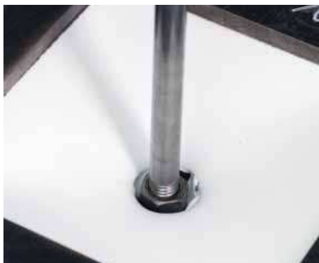
Rigid HDPE perforates when impacted during a puncture test.
