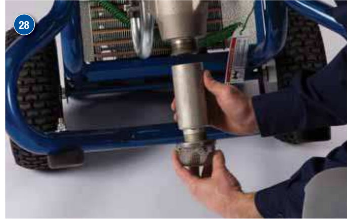
Connect pail adaptor to siphon end of pump.
