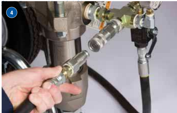
Connect jump hose to Graco pump.
