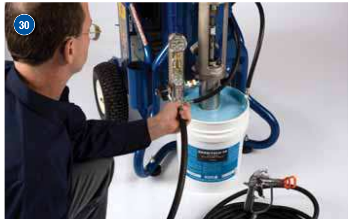
Insert purge line into pail. Connect hose and Graco Silver Gun to discharge of Graco pump.
