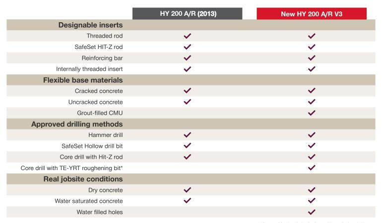
$<sup>{}^\</sup>star\! Approved$  for threaded rod, rebar and internally threaded inserts
