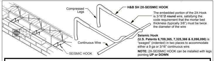
Hohmann & Barnard's 2X-Hook has been tested and designed to withstand over 200-lbf, in tension or compression, at maximum allowed offset (TMS 402/602-16 12.2.2.5.5.4) of 1¼" (disengagement of the pintle from the veneer anchor). These results exceed BIA recommendations and the capabilities of standard "round wire" hooks/pintles by over 100%, while maintaining the ASTM A1064/1064M wire specification. 2X-Hook: U.S. Pat. No. 8,613,175
