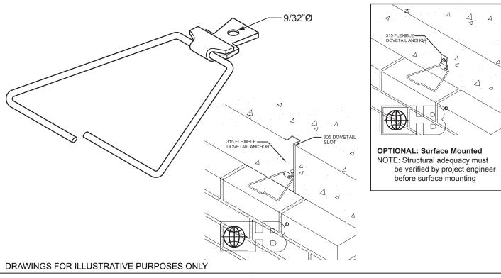
315 Flexible Dovetail Brick Tie permits horizontal and vertical movement of the masonry wall while, restraining tension and compression. For use with 305 Dovetail Slot or surface mounted to concrete or block to block or brick.
