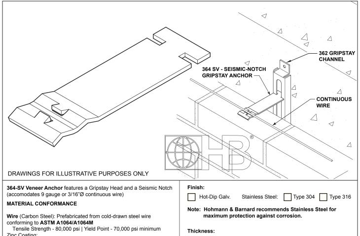
Hot-Dip Galvanized after fabrication: **ASTM A153/A153M-B** (1.5 oz/ft²) Note: Hohmann & Barnard will certify to a minimum of 2.0 oz/ft2
