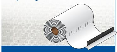
HB BELOW-GRADE 60 is a 60 mil Heavy Duty Self-Adhering Below-Grade Waterproofing Membrane, that features a woven polyethylene membrane coated on both sides with a uniquely engineered waterproofing blend. The polyethylene membrane is bonded to a self-sealing, highly adhesive, bituminous layer protected by a convenient release liner.
