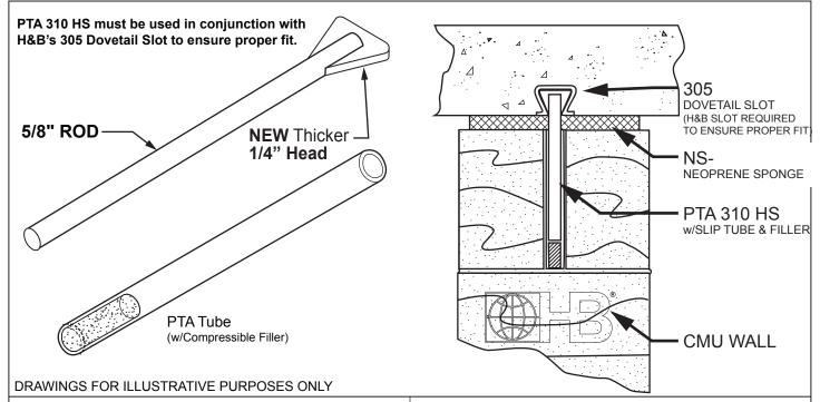
PTA 310 HS provides lateral shear resistance at the upper limit of masonry walls. They permit vertical deflection of the slab above, without transferring compressive loads to the masonry wall below. PTA Series Anchors are suitable for construction using steel or concrete. PTA Tube with expansion filler is placed over rod anchor, which has been attached to concrete or steel. The vertical joint is then filled with mortar, fully surrounding the tube.
