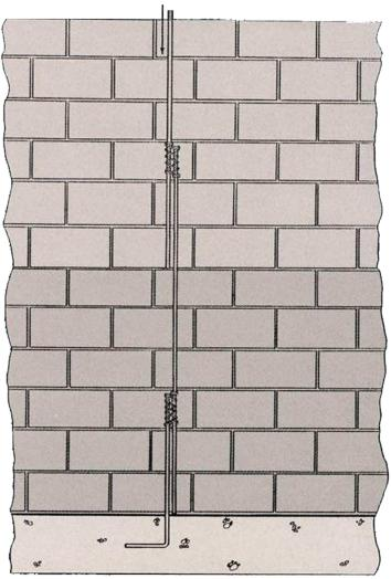
Detail shows completed base and intermediate **SPYRA-LOX™** connection.
