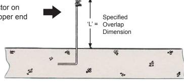
> 2) Build masonry to a height equal to 2 x 'L' (two times overlap dimension)
