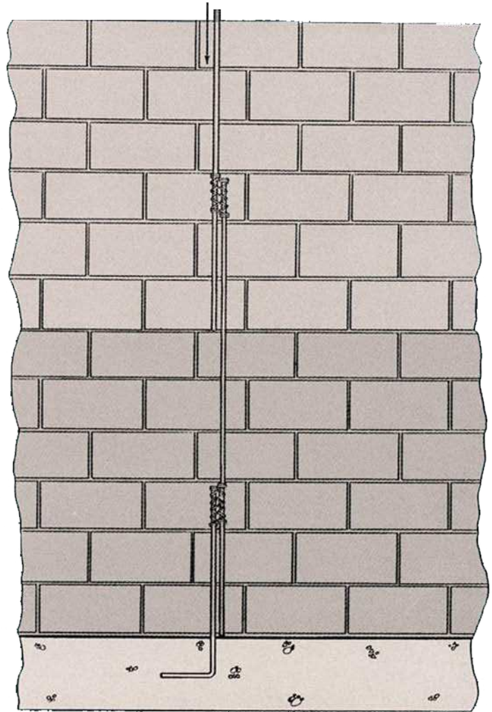
Detail shows completed base and intermediate SPYRA-LOX™ connection.
