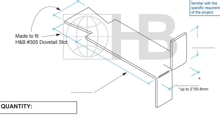
ST/ST Plate Min. Fy. = 45,000 p.s.i. (ASTM A666)
