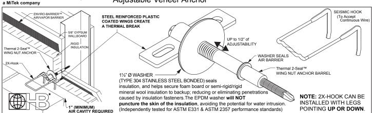
Hohmann & Barnard's 2X-Hook has been tested and designed to withstand over 200-lbf, in tension or compression, at maximum allowed offset (TMS 402/602-16 12.2.2.5.5.4) of 1½" (disengagement of the pintle from the veneer anchor). These results exceed BIA recommendations and the capabilities of standard "round wire" hooks/pintles by over 100%, while maintaining the ASTM A1064/1064M wire specification.
