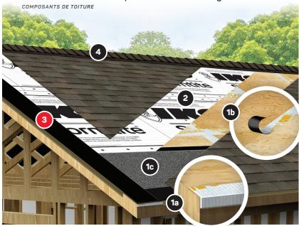
PROTECTION DU PLATELAGE | RUBAN D'ÉTANCHÉITÉ DE TOITURE
