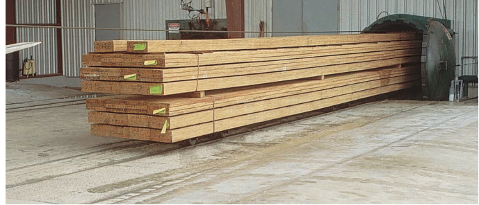
Parallam® Plus PSL products enter an airtight treatment cylinder—a highly controlled, pressurized environment where they are exposed to the treatment process.
