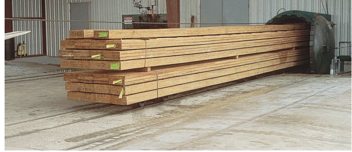
Parallam® PSL products enter an airtight treatment cylinder—a highly controlled, pressurized environment where they are exposed to the treatment process.
