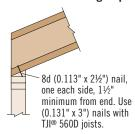
When slope exceeds 14:12, a beveled bearing plate, variable slope seat connector, or birdsmouth cut (at low end of joist only) is required.
