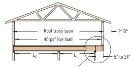
TJI® joists may be cantilevered 5" to 24" when supporting roof load, assuming:
