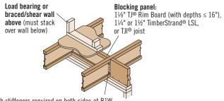
Web stiffeners required on both sides at B1W ONLY. See footnote (1) under span tables.
