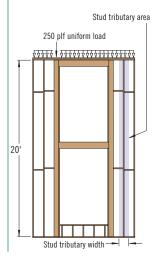
(1) Load based on a wind pressure of  $19.1\ \mathrm{psf}$  and studs spaced at  $16\mbox{"}$  on-center.
