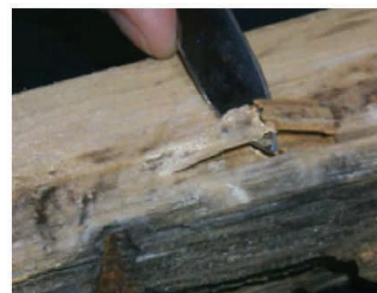
Pick test on decayed wood—brash break
