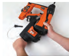
M034 fastener used to hang HVAC Duct Strap
