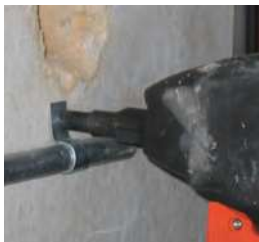
12HSMP034 clip assembly used to secure conduit
