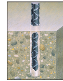
Doweling into Concrete with Rebar
