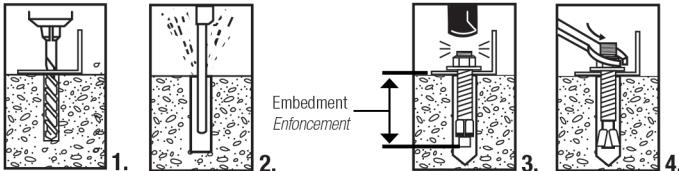
1. Select a carbide drill bit with a diameter equal to the nominal anchor diameter. Drill hole at least 1/4" deeper than nominal anchor embedment.
