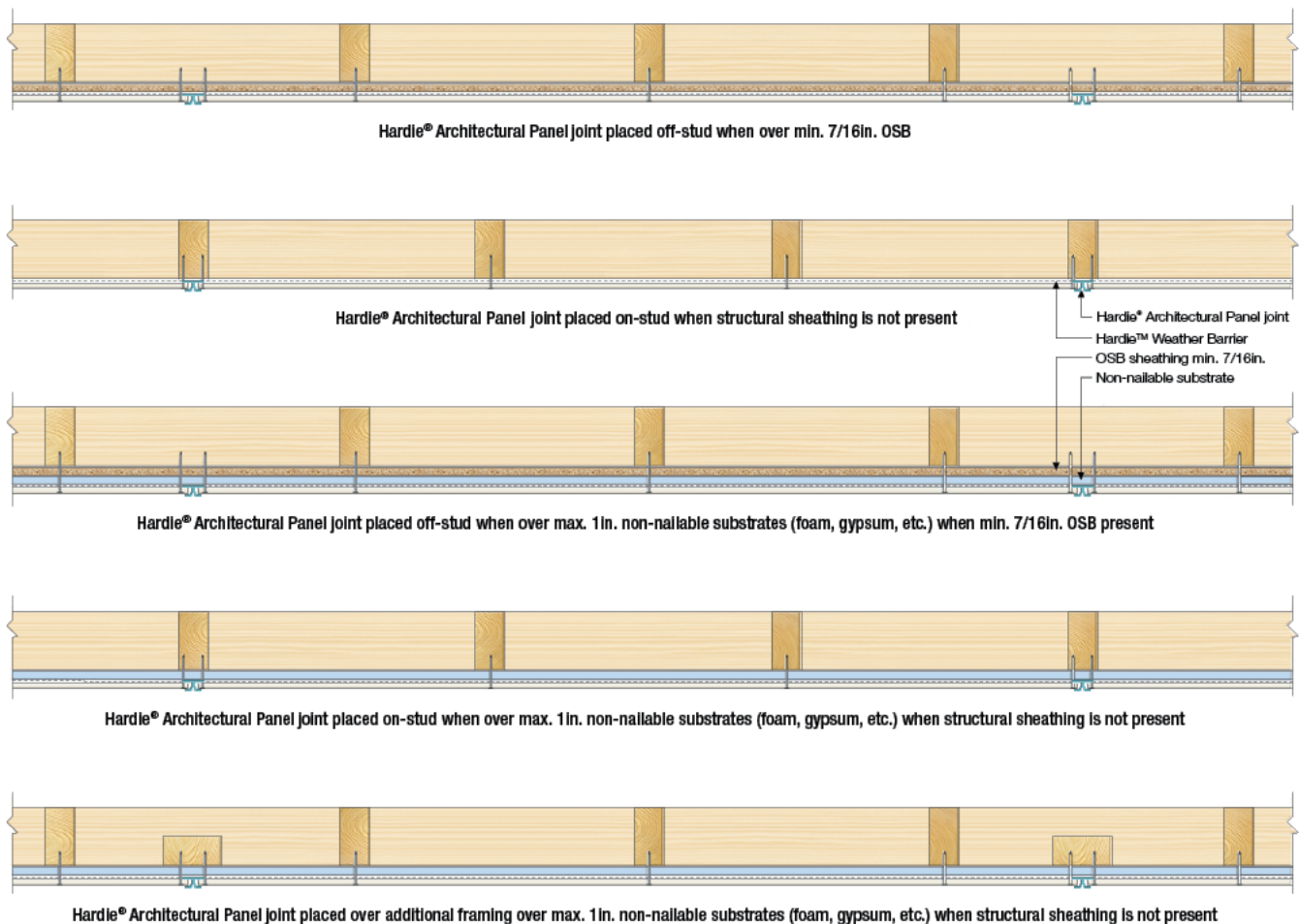
Figure 8.13 - Panel joint placement options
