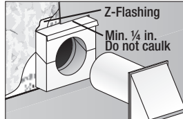
Figure 4.11 Block Penetration (Recommended for HZ10®)
