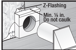
Figure 13 Block Penetration (recommended in HZ10)
