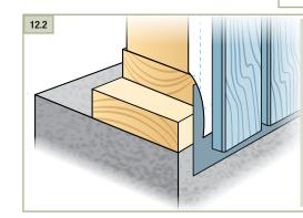
TIP: Install flashing over the footing/foundation and extend the panel over the flashing just below the sill plate. Do not extend siding beyond the required grade clearances. TIP: For Sierra 8 panels, double studs at each panel joint allows fasteners to be placed outside of panel grooves.
