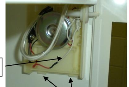
To replace alarm cover - Hook cover on bottom 2 hooks - Then snap top of cover in-place.
