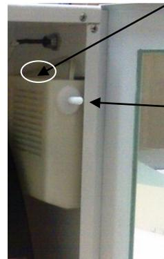
Slot to open alarm enclosure. You can use a flat screw driver or the flat edge of the key to open.
