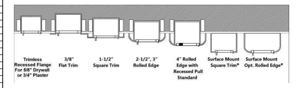
\*Note: for surface mount cabinets, add 3-3/16" to width and height measurements.
