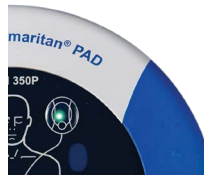
Figure 11. Flashing green LED; no action required.
