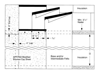
**12.11 Nailable and Lightweight Concrete Decks:** On decks with a slope over ½" per ft (42 mm/m), the roofing felts must be installed parallel to the incline. Nail the end laps of the modified bitumen cap sheet across the width of the sheet on 8½" (216 mm) centers. All nails are to be covered by the lap of the next sheet. For slopes from ½" to 2" per ft (42 to 167 mm/m), a full-length sheet can be used. For slopes from 2" to 3" per ft (167 to 250 mm/m), a half-length sheet should be used.
