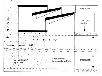
12.5 Nailable and Lightweight Concrete Decks: On decks with a slope over  $2\frac{1}{2}$ " per ft (208 mm/m), the roofing felts must be installed parallel to the incline. Nail the end laps of the modified bitumen cap sheet across the width of the sheet on  $8\frac{1}{2}$ " (216 mm) centers. All nails are to be covered by the lap of the next sheet.
