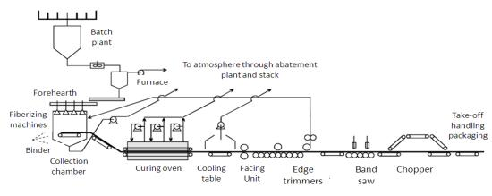
Figure 3: Manufacturing process steps
