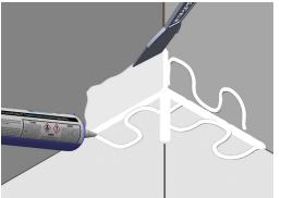
2. Apply 1/4" beads of sealant in a ribbon pattern spaced 1 to 2" apart within extents of GoBoard Corner. 3. Spread sealant with a putty knife slightly beyond extents of GoBoard Corner while ensuring joints are filled with sealant.
