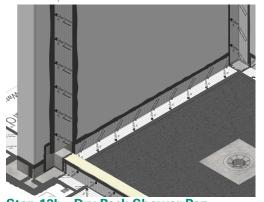
**Step 13b - Dry Pack Shower Pan** For dry pack pans using GoBoard Point Drain System, install GoBoard Corner, Curb Cover then Banding around perimeter as shown.
