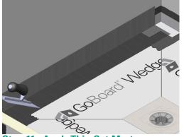
**Step 11 - Apply Thin-Set Mortar** Comb thin-set beyond extents of banding using a 3/16-in. x 5/32-in. v-notch trowel. Include at least a 2-in. overlap with accessories and membrane.
