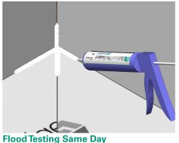
Use GoBoard Pro Sealant or GoBoad Sealant in place of thin-set mortar. 1. Liberally fill joints with sealant within extents of GoBoard Corner.
