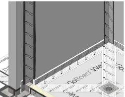
extents of banding, **3**. Spread sealant with a putty knife, **4**. Embed banding into sealant, **5**. Ensure full coverage and squeeze out excess sealant. This procedure can also be used for dry pack shower pans when dry prior to installing topical waterproofing.
