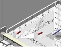
**Step 13c - Flood Testing Same Day** See previous steps for flood testing same day. **1.** Fill joints with GoBoard Sealant or GoBoard Pro Sealant, **2.** Apply 1/4-in beads spaced 1 to 2-in apart within
