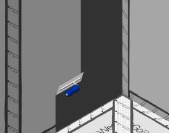
**Step 15 - Apply Thin-Set Mortar** Uniformly apply thin-set mortar with a 3/16-in x 5/32-in v-notch trowel accounting for 2-in overlap with banding, corner, curb cover and membrane.
