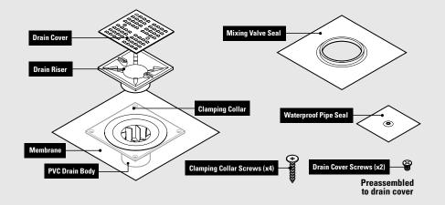
**NOTE:** The GoBoard Point Drain shower pan system accomodates all types of shower areas and offset drain locations, so there's no need to move the existing plumbing.
