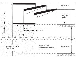
**8A.12.5** Nailable and Lightweight Concrete Decks: On decks with a slope over  $2\frac{1}{2}$ " per foot (208 mm/m), the roofing felts must be installed parallel to the incline. Nail the end laps of the modified bitumen cap sheet across the width of the sheet on  $8\frac{1}{2}$ " (216 mm) centers. All nails are to be covered by the lap of the next sheet.
