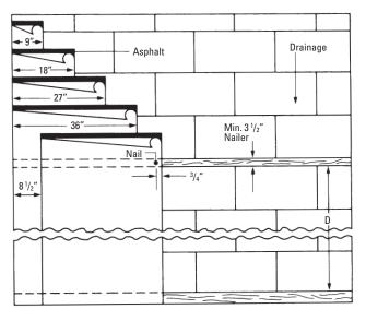
Nailing Pattern and Nailer Spacing shown with Cap Sheet Roofs.
