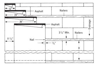
Nailing Pattern and Nailer Spacing shown with 4-Ply System.
