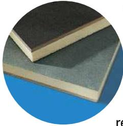
⊕ **Fesco Foam**® is a rigid insulation board for use over metal, nailable and non-nailable decks in BUR, modified bitumen and certain single ply roofing systems. It is composed of a polyisocyanurate foam core, bonded to a ½ inch (127 mm) Fesco laminator board on one side and a universal fiber glass-reinforced facer on the other.
