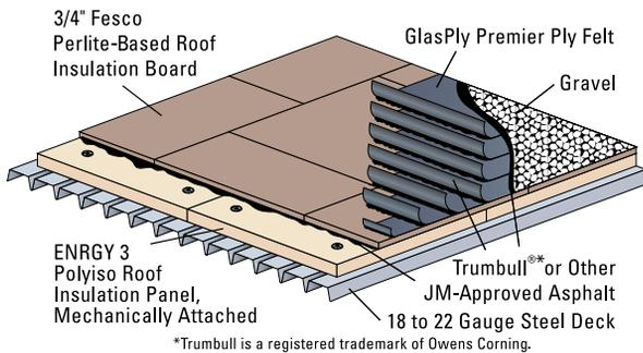
**Four-ply, gravel-surfaced, fiber glass built-up roof. For use over JM insulation, approved decks or other approved insulations, on inclines up to 3 inches per foot (250 mm/m).**
