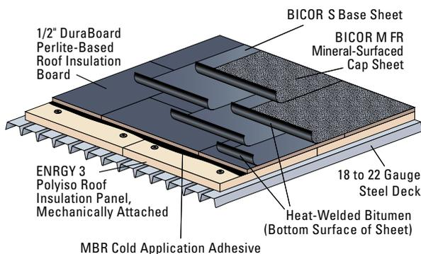
**Two-ply, heat-welded, modified bitumen, mineral-surfaced roofing system. For use over JM insulation, approved decks or other approved insulations on inclines up to 6 inches per foot (500 mm/m).**
