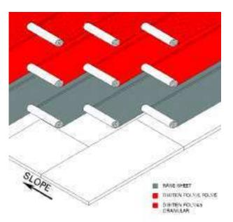
bleedout of compound shall be visible at the edge of all seams. All laps must be checked for good adhesion. Preparation of the 6" (152 mm) end lap requires scuffing away all loose granules. Heat and embed all remaining granules. Apply heat to the roll being seamed while making sure both have a good compound flow to adhere the two surfaces. End laps must be checked for proper adhesion.
