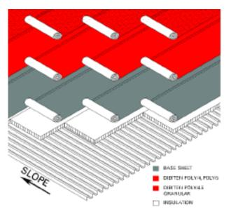
mm) wide piece of base ply through the insulation. The remaining base plies are to be applied full width with 3" (76 mm) side and 4" (102 mm) end laps over the preceding sheets. Fasten the laps at 9" (229 mm) centers, and down the longitudinal center of each felt ply, place two rows of fasteners, with the rows spaced approximately 11" (279 mm) apart, and fasteners staggered on approximately 1/8" (457 mm) centers. Use fasteners appropriate to the insulation and deck.
