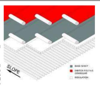
with 3" (76 mm) side and 4" (102 mm) end laps over the preceding sheets. Fasten the laps at 9" (229 mm) centers, and down the longitudinal center of each felt ply, place two rows of fasteners, with the rows spaced approximately 11" (279 mm) apart, and fasteners staggered on approximately 1/8" (457 mm) centers. Use fasteners appropriate to the insulation and deck.
